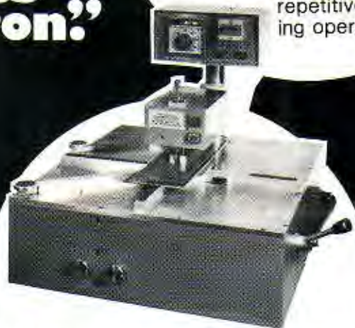
Multicore Solderability Testers. MK III - Tests components semi-automatically. New PTH - tests plated-through-holes in P.C. boards automatically.
